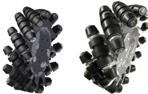
Figure 3 Mecanum Wheels (a) CAD Design (b) Final Product
